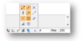
Snapping the end points of graphical (lines, arcs) and structural (beams, columns) objects
