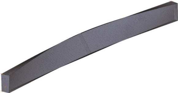
Fig. 7. Global stability analysis by Shell3 model ( \alpha_{cr}=1,40 )
