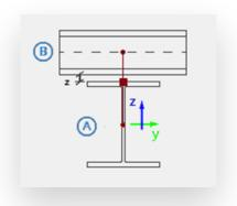
The link elements can be placed individually or in groups with a predetermined arrangement along the main beam.
